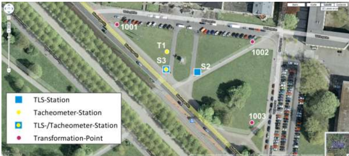
Figure 1: Configuration of the practical experiment in front of the Leibniz Universität Hannover (Image by Google Maps)
