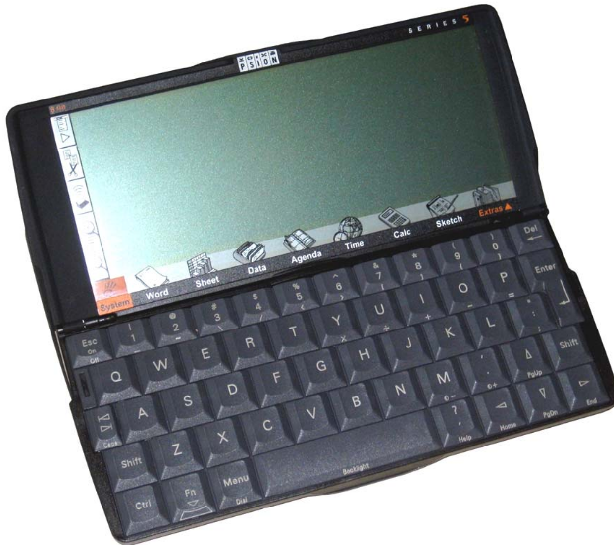
Psion Series 5 Handheld-Computer 32-Bit ARM 710 (18,432 MHz) ROM 6 MB, RAM 4 MB/8 MB
